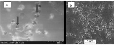
Fig.1. Microstructure of DMV 617 mod: a)  $\gamma'$  phase precipitates (arrows) and b)  $M_{23}C_6$  carbides
