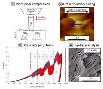
Figure 1 Techniques utilized in the investigation of deformation mechanisms in biodegradable ultrafine-grained Zn alloys
