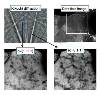
Fig. 1. An example of two dislocation images reconstructed from Kikuchi diffraction patterns recorded in the region marked by the white rectangle in the dark-field image.
