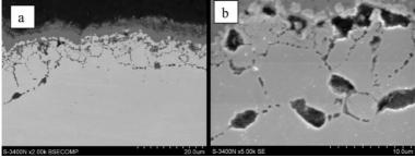
Fig.2. Oxidation products resulting from corrosion in a steam environment include: a) a  $Cr_2O^3$  oxide layer on the surface and b) an internal oxidation zone.
