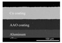
Fig. 1. Structure of the AAO-Cu coating.
