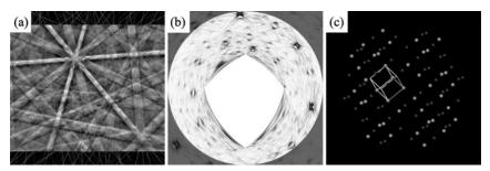
Fig.1. Key stapes of the CALM analysis: a) experimental pattern with marked traces of crystallographic planes b) Funk transformation c) reciprocal lattice with the unit cell for the experimental pattern
