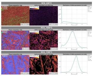
Figure 1. Phase composition maps, lattice parameters (c/a) distribution maps and distribution of the lattice parameters for NC6 steel after different austenitization temperatures for 30 minutes
